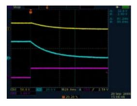
Figure 2. Output Voltage After Switch Off
