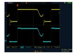
Figure 8. Switching Waveforms
