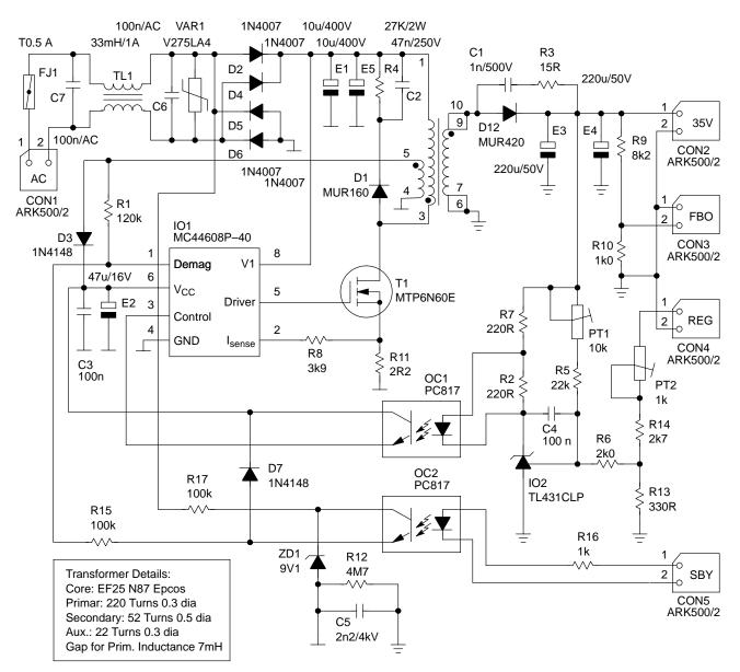
Figure 1. Schematic of SMPS
