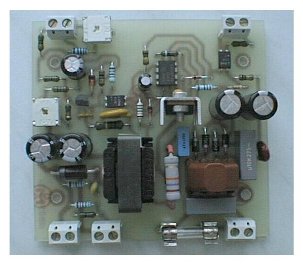
As it is well known, according to power saving regulations, we need to obtain a very low power consumption during standby condition for all equipment continuously powered on the mains. For "not saving" version of power supply, the standby power consumption is around 9.0 W (for 100 W power output). When using the MC44608 GreenLine<sup>™</sup> Power supply controller, we obtain 1.3 W in standby mode. The result is absolutely phenomenal, but still, for some special applications, the
